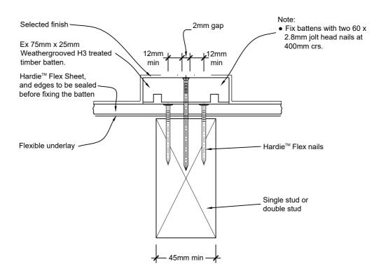
Alternatively an Axent  $\!^{\text{\tiny TM}}$  Trim with two 6mm continuous beads Bostik Seal N Flex-1 can be used.
